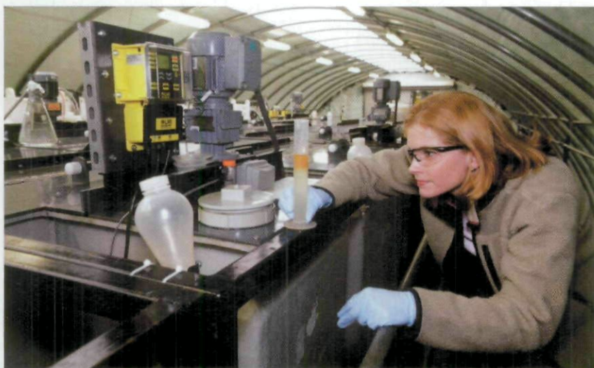
A test facility in Pennsylvania treats ARD at a rate of 30 gpm.
